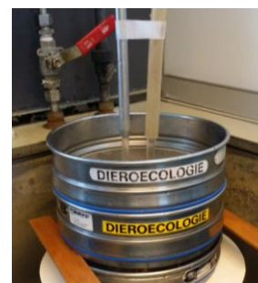
Figure 2 Three stacked sieves with descending mesh sizes were used to filter microplastics out of plain river water.
