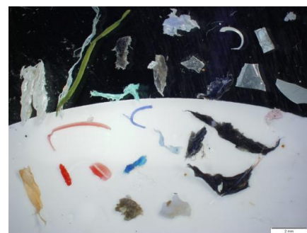
Figure 14. Examples of the group of so called miscellaneous MPs, in the size range 0.250-5 mm observed in Rhine river sample L16. Scale bar = 2 mm
