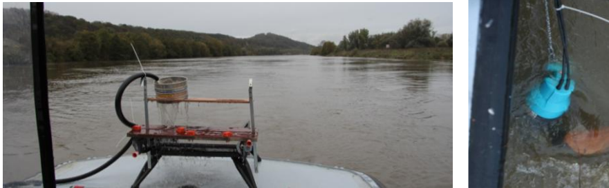
Figure A3. Pilot sampling in the mid section of the river Meuse (Eijsden) using a submersible pump. (a, left) Water was directly led over the sieves. Water could run freely through a hole in the hardboard plate. (b, right) Position of the submersible pump just below water surface.
