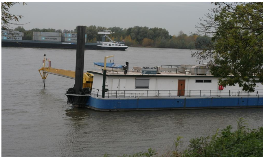
Figure 1. Monitoring station at Lobith (Rhine). The station at Eijsden is similar. Water is taken in permanently by the yellow crane jib and released at the other front. Several taps are available for analytical purposes, of which one was reserved for this study on microplastics.
