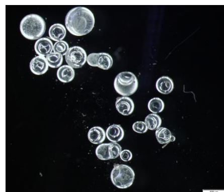
Figure 17. Examples of transparent spherules > 0.250 mm found in the Rhine river (sample L16). Scale bar = 0.5 mm
